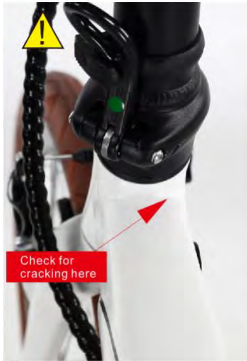
Check the head tube junction for fatigue cracking
