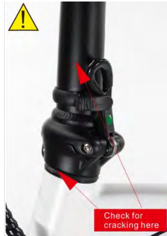
Check the head tube junction for fatigue cracking
